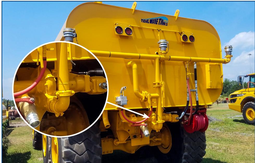
101-B69875 Pump shown here on an 8,000 Gallon, Volvo A40G Tank System
