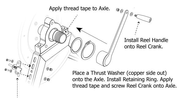
Install Reel Lock onto Frame using two 5/16-18 x 7/8" bolts, four 5/16" washers and two 5/16" nuts. Line up the Reel Lock pin with the Locking Hose Guide holes. Crank the reel a full turn to ensure it does not rub on the Hose Guide. Adjust if needed, then tighten bolts on the Reel Lock and Assemblies.
